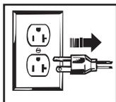
**DE-ENERGIZE, DISCONNECT AND LOCK OUT ALL POWER SOURCES DURING MAINTENANCE**
