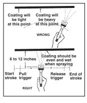
For best results, use 3 to 6 psi fluid pressure. Higher than 6 psi fluid pressure may be required for heavy-bodied materials. Low fluid pressures will produce a narrower than normal spray pattern. Generally use 30-35 psi air at gun inlet (see page 7). Unusually heavy, difficult to atomize fluids may require up to 50 psi air at gun inlet.
