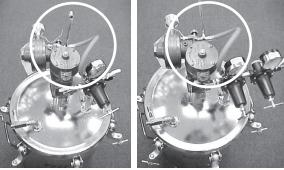
Assemble hose to either manifold using a 5/8 wrench.
